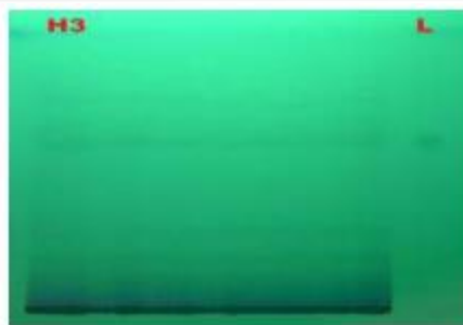
Figure 3. PLC plate showing the detected luteolin band under UV at 254 nm. Developed in mobile phase S1 (Ethyl acetate: Formic acid: Hexane). H3: ethyl acetate fraction, L: luteolin standard.
